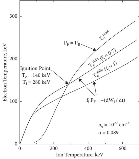
FIGURE 2: Ignition points in the  $T_e$ - $T_i$  plane for high-density H- $^{11}\text{B}$  plasma.  $f_i$  is the fraction of fusion power to plasma ions;  $\alpha$  is the boron-to-proton ion concentration. Reproduced from Moreau [9] with the permission of the publisher. © IAEA 1977.
