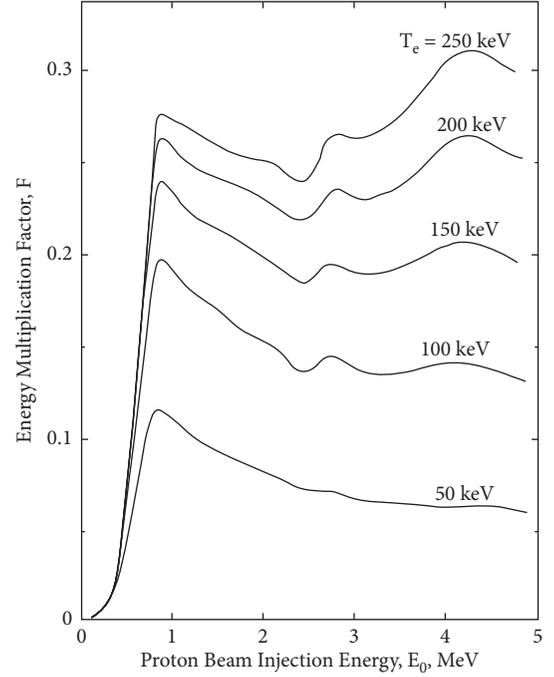
FIGURE 6: Energy multiplication factor vs proton injection energy for various electron temperatures. Protons are injected into a <sup>11</sup>B plasma with cold ions and warm electrons. The results are independent of plasma density when the value of  $\ln\Lambda$  is fixed. Reproduced from Moreau [9] with the permission of the publisher. © IAEA 1977.
