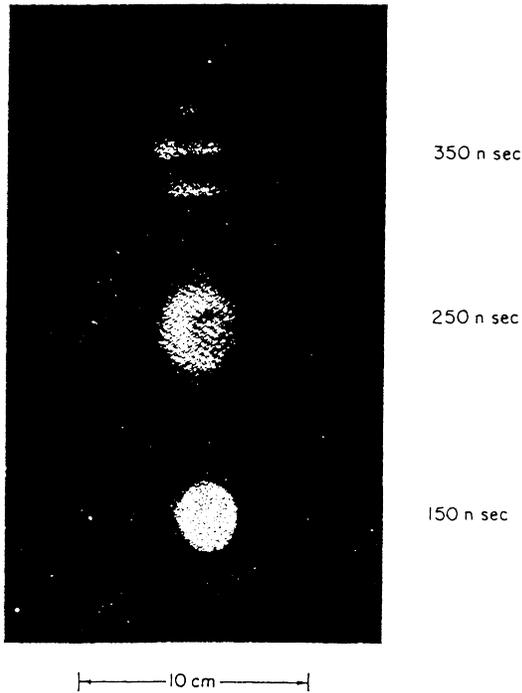
**Fig. 1.** Side-on framing camera picture of a plasma produced from an aluminum sphere of  $80 \mu\text{m}$  radius at the time indicated after irradiation by a  $30 \text{ ns}$  ruby laser pulse focused to  $0.4 \text{ mm}$  diameter. The second frame shows the outer part of a rapidly expanding plasma and an inner spherical thermally expanding part [13][14].
