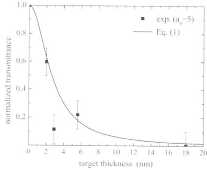
Fig. 5. Points are the transmission laser energy incident of 810 nm wave length CPA pulses of 1.2 J and 45fs duration per incident laser energy at a diameter of 3.6  $\mu\text{m}$  of diamond layers of varying thickness [41] (with permission of the publisher).
