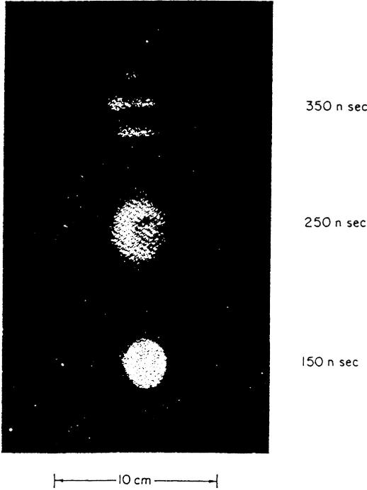
*Fig. 1. Side-on framing camera picture of a plasma produced from an aluminum sphere of 80  $\mu\text{m}$  radius at the time indicated after irradiation by a 30 ns ruby laser pulse focused to 0.4 mm diameter. The second frame shows the outer part of a rapidly expanding plasma and an inner spherical thermally expanding part [13][14].*
