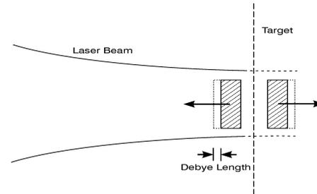
**Fig. 3.** Scheme of skin depth laser interaction where the non-linear force accelerates a plasma block moving against the laser beam and another block towards the target interior as a kind of dielectric explosion. In front of the blocks are electron clouds of the thickness of the effective Debye lengths for the conditions of Fig. 2
