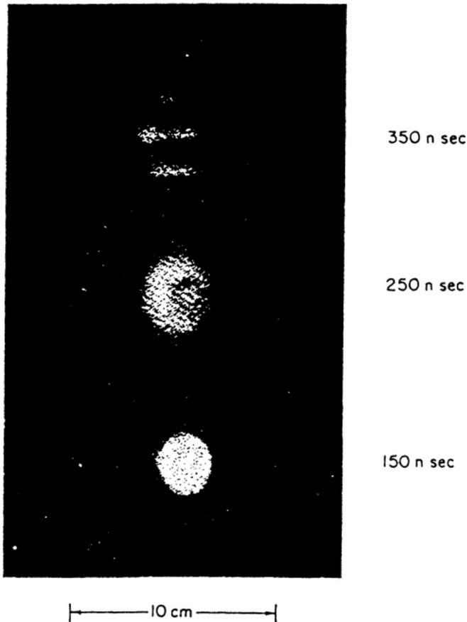
Fig. 1. Side-on framing camera picture of a plasma produced from an aluminium sphere of 80  $\mu\text{m}$  radius at the time indicated after irradiation by a 30 ns ruby laser pulse focused to 0.4 mm diameter. The second frame shows the outer part of a rapidly expanding plasma and an inner spherical thermally expanding part [13,14].
