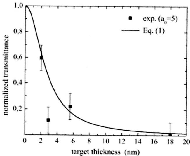
Fig. 5. Points are the transmission laser energy incident of 810 nm wave length CPA pulses of 1.2 J and 45 fs duration per incident laser energy at a diameter of 3.6  $\mu\text{m}$  of diamond layers of varying thickness [40] (with permission of the publisher).
