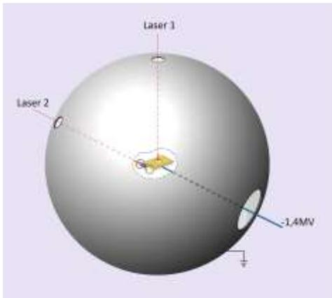
**Fig. 1.** Schematic of a boron-fusion reactor and electric power generator, which generates low-cost energy and does not produce dangerous nuclear radiation [21][22][23]. The reaction unit in the center is described in Fig. 2.
