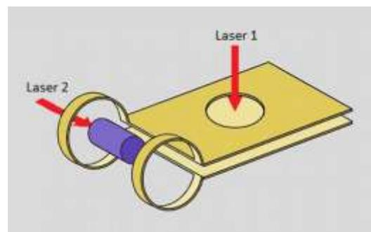
**Fig 2.** Reaction unit in the centre of the reactor of Fig. 1 using “capacitor coil fields” producing a cylindrical magnetic field of kilotesla magnitude [24]. The cylindrical target with the HB11 fuel is co-axially located in a coil where, for a ns, the kilotesla magnetic field is produced by a kJ-ns laser pulse 1. A ps-30kJ laser pulse 2 initiates the
